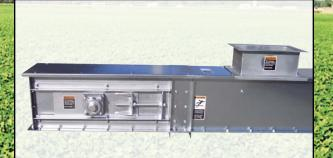
Acme screw take-up assembly on tail section, bearings outboard mounted with UHMW dust seals. Standard inlet with UHMW V-splitter over chain to reduce chain wear.
