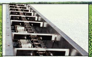
UHMW paddles are bolted onto steel attachments that are welded onto a heavy duty steel chain, factory installed in 10' sections with (4) UHMW return chain rollers.
