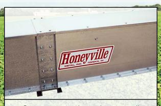
Conveyor trough sections are all G-90 formed galvanized steel with no welding on any exterior panels. Bolted formed channel type trough connections.
