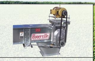
Head and tail sections G-90 galvanized steel, all sprockets with taper lock bushings. Class II Dodge torque-arm type gear reducer installed with over-head motor mount and fixed pitch v-belt drives.
