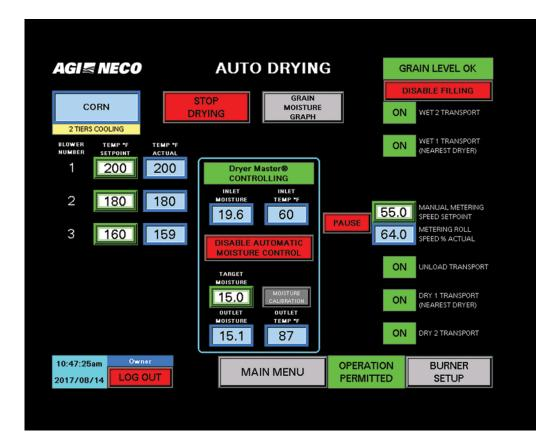
DRYER MASTER provides high quality moisture control in the industry. DRYER MASTER's model based moisture control technology is embedded in NECO's control panel, which is a NECO EXCLUSIVE. Dual moisture sensors provide the information required to deliver accurate, consistent moistures, reduce over and under drying, maximize throughput and lower energy consumption.
