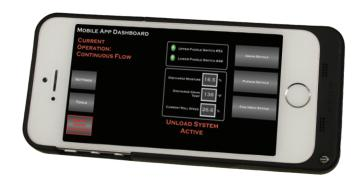
The **GSM PHONE MODEM** works with *QuadraTouch Pro™* controls and operates through GSM cell phone service. If the dryer shuts down, the GSM service sends a text message to a predetermined cell phone number, noting what the fault was. You can also text message the dryer and it will reply with current status, moisture, unload speed and temperature.
