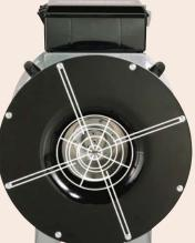
Fan's **air inlet orifice** uses an innovative design to promote better airflow into the centrifugal wheel to enhance fan performance. The unique **baffle** design helps to direct air into the centrifugal wheel to encourage smooth, efficient fan operation. A 10-mil PVC coating on **screen guard** provides an attractive appearance and superior corrosion resistance.
