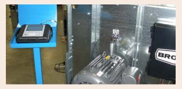
As a part of Brock's high standard of quality and reliability, all GUARDIAN® Series Centrifugal Fans are factory-tested for fan balance to minimize performance-robbing vibration.
