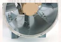
**Air vanes** are a standard feature on all 18-inch (457-mm) diameter and larger fans. The vanes aid efficient airflow at higher static pressures by reducing air turbulence.
